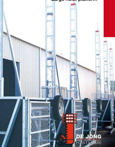
The AT30L is a compact and versatile hoist capable of lifting 300kg with a single phase motor and ideal for sites where power supply is limited. It is easy to transport with a removable tilting system; compact enough to install into a small area; and offers a large platform.
